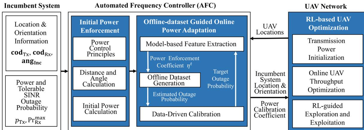
Fig. 2. Diagram of the *SwarmShare* spectrum sharing framework.
