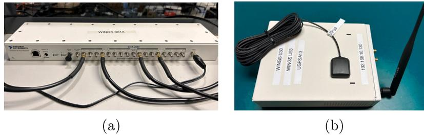
Fig. 10. (a) Snapshot of the Octoclock; (b) GPS module.
